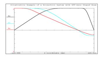
The three principal paraxial rays used to compute the optical properties.
