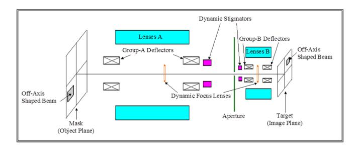
Schematic structure of an electron or ion beam projection system, with an off-axis shaped beam. The two groups of deflectors (Group-A and Group-B) act as aberration-reduction elements
