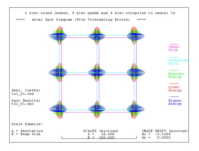
Aberration spot diagram with tolerancing errors
